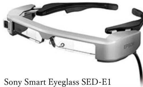
EPSON MOVERIO BT-300 micro-OLED 1,280 x 720
